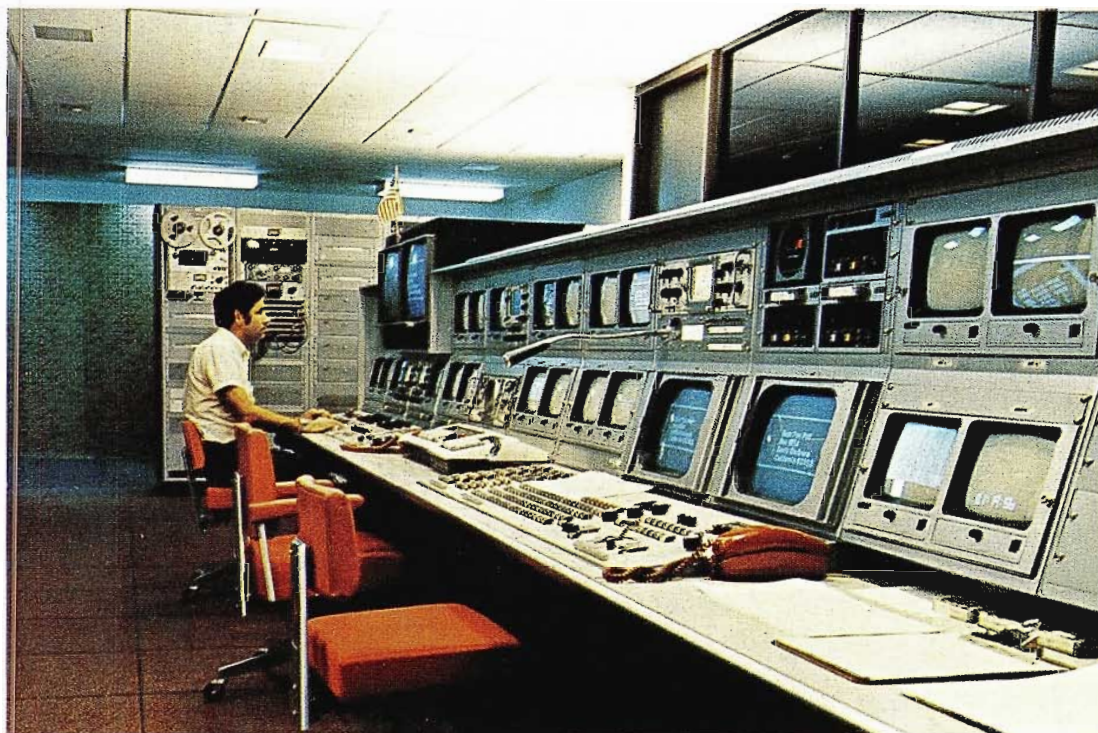
The Master Control console is designed to double as a production position. Assistant Chief Engineer John Jackson shades cameras at far end of console. MC Switcher is in foreground, with Video IV character generator keyboard in center area.
