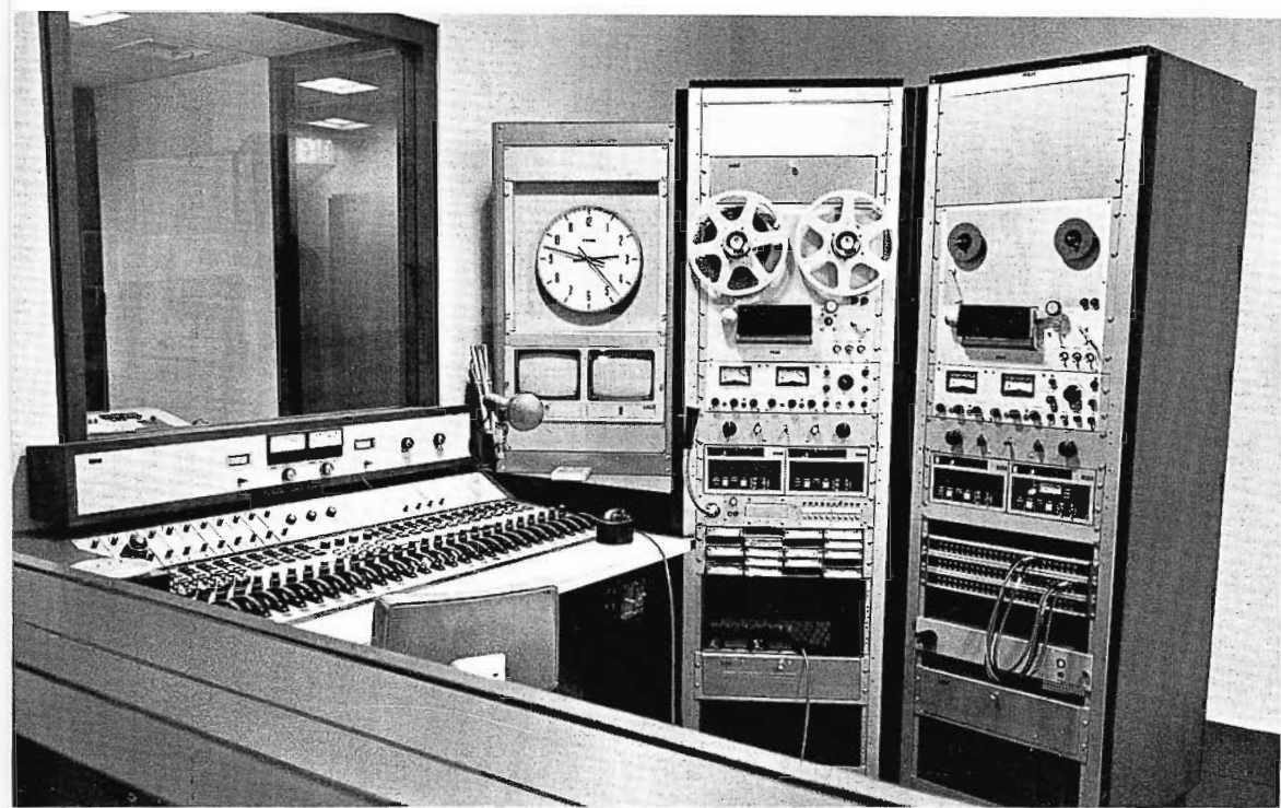
Each studio has a separate audio control room, with audio reel-to-reel and cartridge recorders and a custom BC-100 audio control console.
